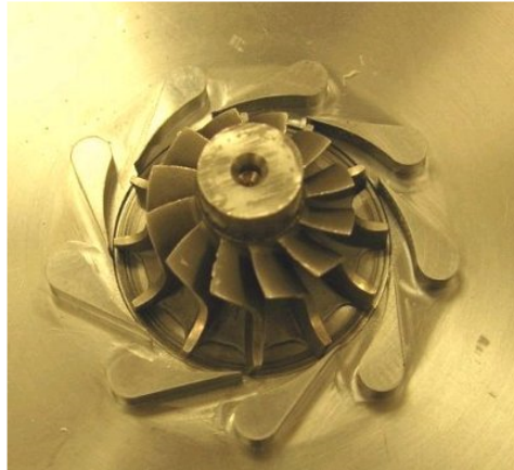
In the Sandia system, the reactor heat is transferred to a very efficient supercritical CO 2 turbine to produce electricity. This turbine wheel was developed by Barber Nichols for Sandia's Brayton experiments.
